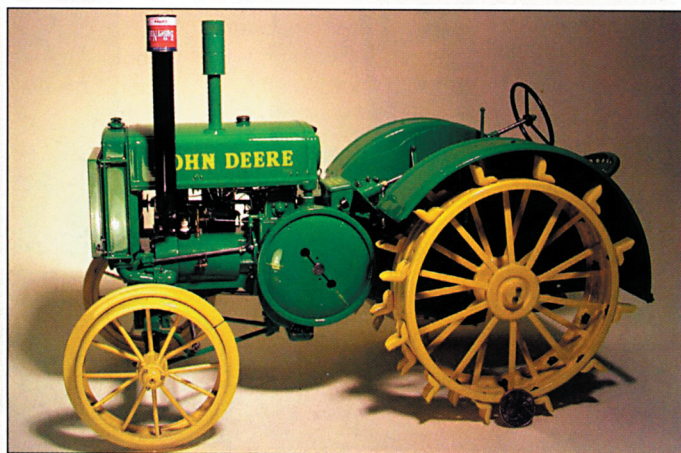
Replica in 1/8 scale of the John Deere D. Note the tiny Butternut coffee can—a low-tech but effective way to keep rain out of the exhaust pipe in the old days. (Photo courtesy of Forrest Atkinson.)
