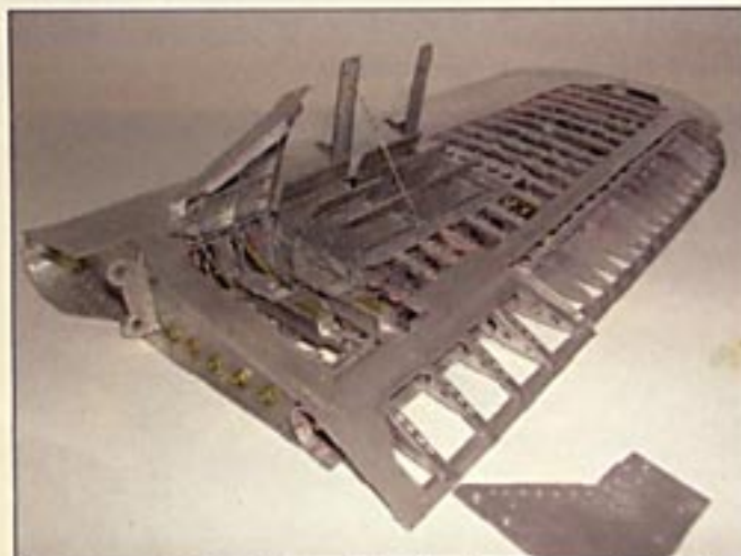
The wings are built from aluminum sheet formed into spars, ribs, and skin panels. The doors over the machine-gun bays are hinged.
