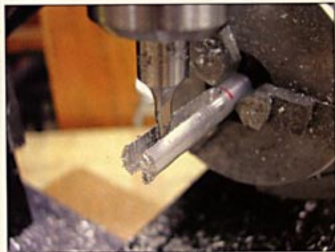
Fashioning the prop blades from aluminum billet is a process of gradual shaping with a milling machine.
