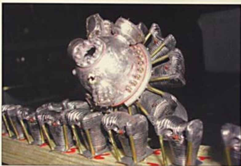
Each cylinder of the R-2800 engine was milled separately.
