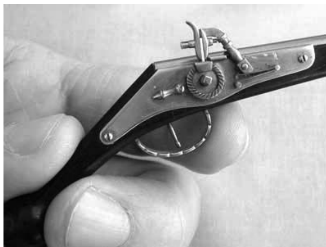
Left & above: A 1/6 scale 16th Century British wheel lock pistol, and a detail of the firing mechanism. The gun consists of 56 separate parts. Completed in 2002, the gun won a prize at the 2004 China International Folk Art Treasures Festival and the 2nd Zhong Hua (TianJin) Folk Art Treasures Exposition. The pistol is complete with a presentation case and tools needed to load and fire the weapon.
