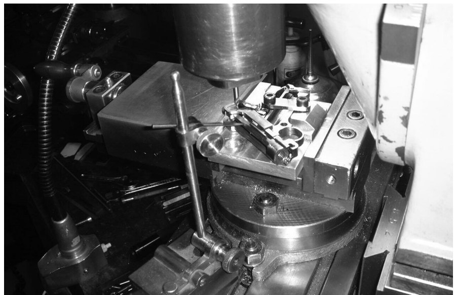
Below: Machining operation on the frame mounted on a special jig. ( 2 were required )
