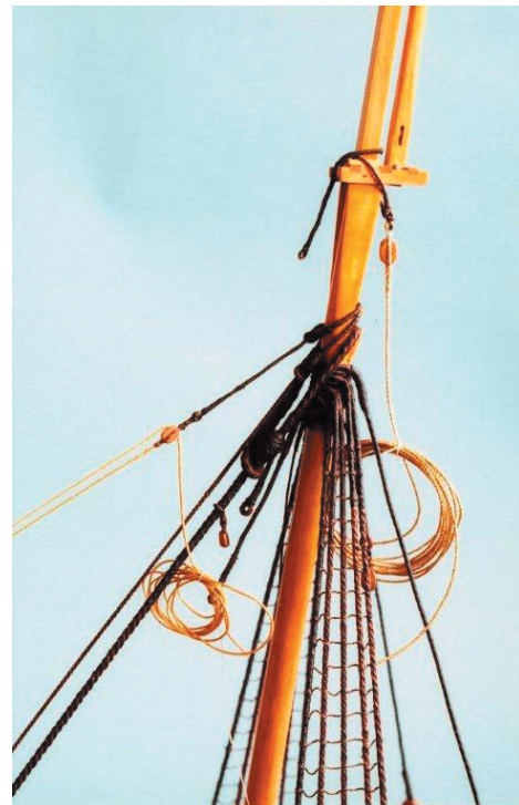
N.R. Cole Photo # 521-16A. Standing and running rigging and masthead details. On the early cutters the topgallant mast was stepped aft of the lower mast as shown here, not in front of it as was common on all but the early cutters and a possibly a few other craft. The line coils were installed while the spars were off the vessel, making things easier later.
