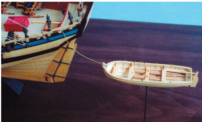
N.R. Cole Photo # 573-01. This view provides a look inside the longboat with her gear stowed and secured for passage.
