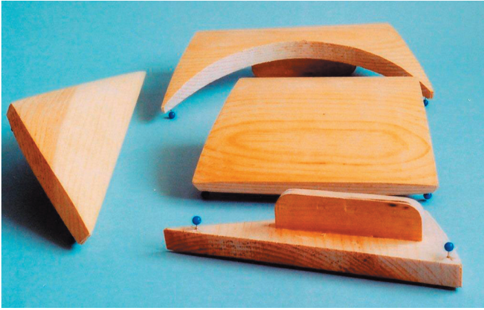
N.R. Cole Photo # 558-24. Carved pine formers over which the sails were moulded into shape.
