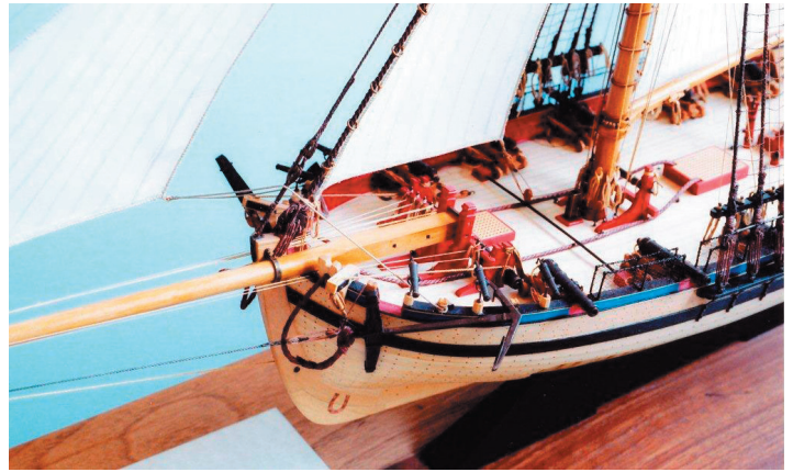
N.R. Cole Photo # 558-06M. Lines from the bowsprit are belayed to pins in the racks across the forward side of the windlass. These lines are led aft to the racks through Lignum Vitae fairleads mounted on either side of the stem and bowsprit. Lines can also be seen belayed to the shroud-mounted pin racks.
