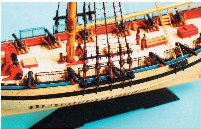
N.R. Cole Photo # 521-07A. This view shows the belaying pin racks installed on the shrouds. Also seen is some of the standing rigging, including the shrouds, ratlines and deadeyes.
