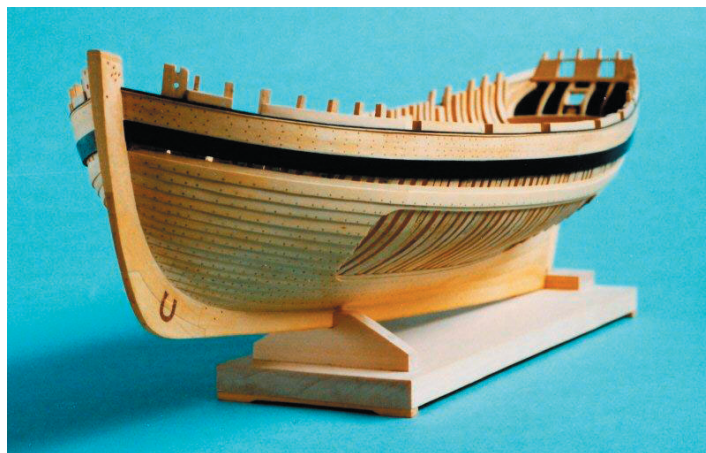
N.R. Cole Photo # 405-19. This photo shows the clenched lap planking with the cutout left open to reveal the framing detail.
