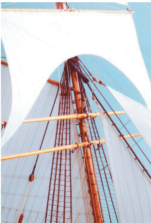
N.R. Cole Photo # 557-02. A wealth of detail, including the mast hoops seized to the luff of the mainsail. The hanks securing the foresail to the forestay can also be seen.
