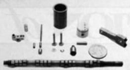
Basic internal components include an accurate, scale duplicate of a Chevrolet performance camshaft, solid lifters, valve seats and guides, valve retainers and locks, cylinder liners, pistons, pins, and aluminum connecting rods.
