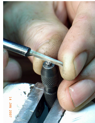
(Above) Cutting screw slots with fine toothed saw.
