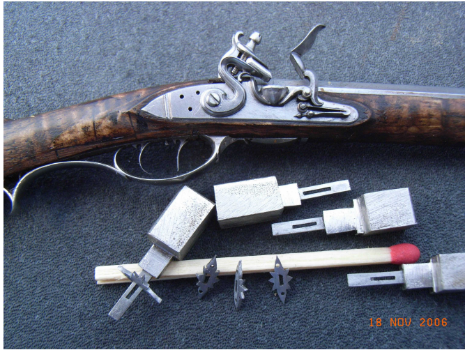
Rifle with dummy stock, barrel key blanks and roughed out escutcheons.
