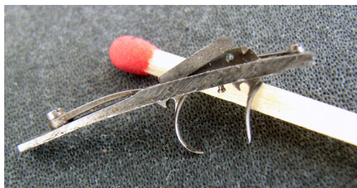
Set triggers at rough filed stage.
