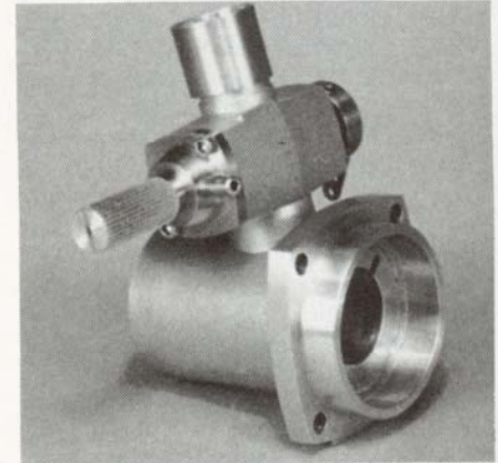
Left and right side views of carburetor/front housing assembly. Two needle type carburetor design worked flawlessly.
