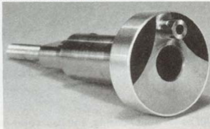
LEFT: Counterbalance end of crankshaft showing molded plastic "case stuffer" inserts (see text). RIGHT: Two piece head assembly. Note unusual treatment given to the head fins. Separate head "button" has flat bottomed combustion chamber with unusually steep angled squish band. Helicopter head uses same combustion chamber button.
