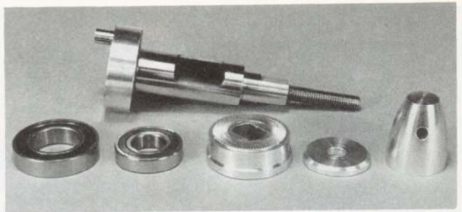
LEFT: Piston, wrist pin, and rod assembly. Small cut-out in piston aligns with sleeve boost port for piston cooling and mixture transfer. Con-rod bronze bushed at both crank pin and wrist pin ends with both ends sharing the same inside diameter. Note position of lubrication holes (see text). RIGHT: Crankshaft, bearings, and prop drive parts. Prop drive washer driven by flats on crankshaft eliminates the chance of drive collet slippage or loss of drive key.
