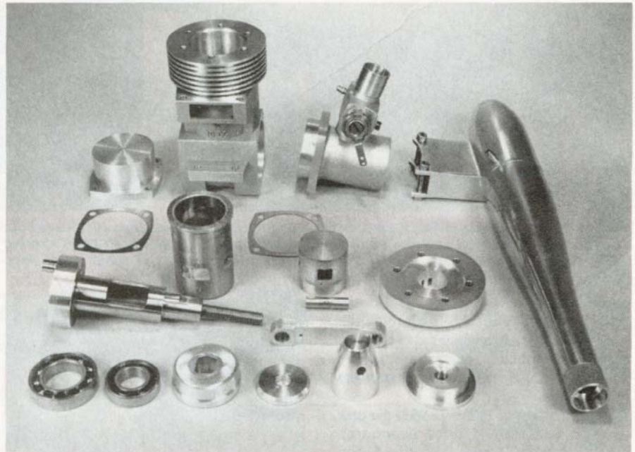
All parts, front housing, and backcover gaskets are made of copper and not paper.
