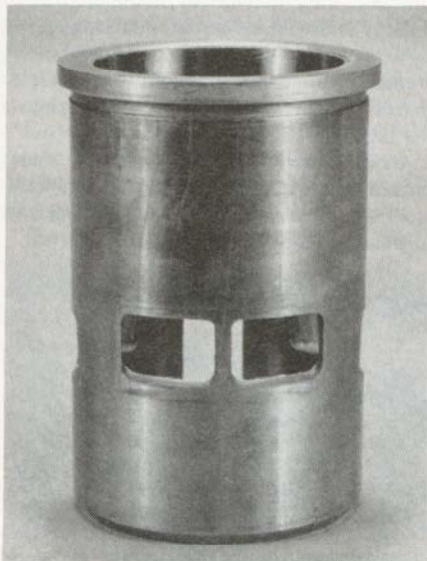
Front, side, and rear views of cylinder sleeve. A large and small side transfer port used in conjunction with a small rear boost port. Seven ports in all.
