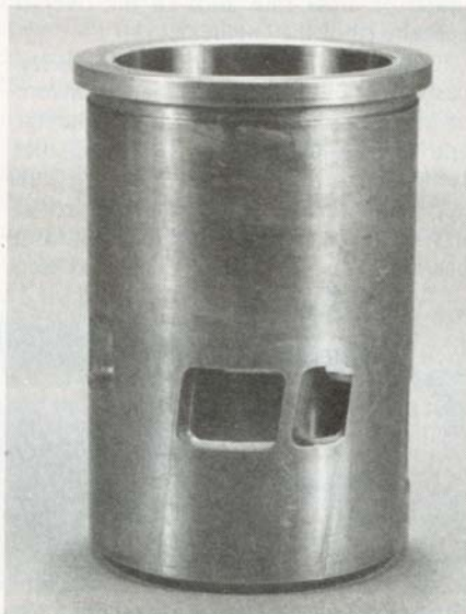
Front, side, and rear views of cylinder sleeve. A large and small side transfer port used in conjunction with a small rear boost port. Seven ports in all.
