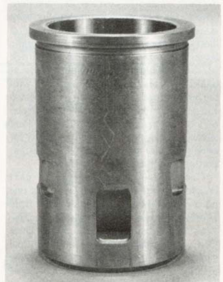
Front, side, and rear views of cylinder sleeve. A large and small side transfer port used in conjunction with a small rear boost port. Seven ports in all.
