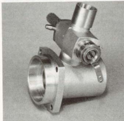
Left and right side views of carburetor/front housing assembly. Two needle type carburetor design worked flawlessly.
