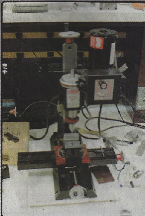
Just one of the Sherline machines available to hobbyists. This is an 8 direction mill, Model 2000.
