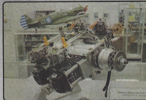
This is a flat four model airplane engine with four independent carburetors controlled by one linkage. Would you believe the cylinder assemblies are from Honda weed eaters?
