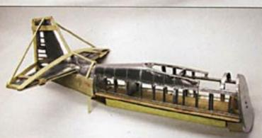
■ Using a wood buck, Young constructed the fuselage in separate pieces, beginning with the tail and moving toward the nose.
